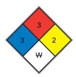
Short exposure could cause serious temporary or moderate residual injury (e.g. <u>liquid hydrogen, sulfuric acid, calcium hypochlorite</u>, hexafluorosilicic acid)
