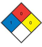
HEALTH 1 Exposure would cause irritation with only minor residual injury (e.g. acetone, sodium bromate, potassium chloride)
