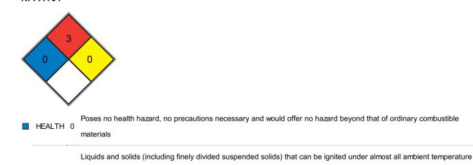
■ REACT 0 Normally stable, even under fire exposure conditions, and is not reactive with water (e.g. helium, N2)
