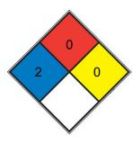
Materials that will not burn under typical fire conditions, including intrinsically noncombustible materials such as concrete,
